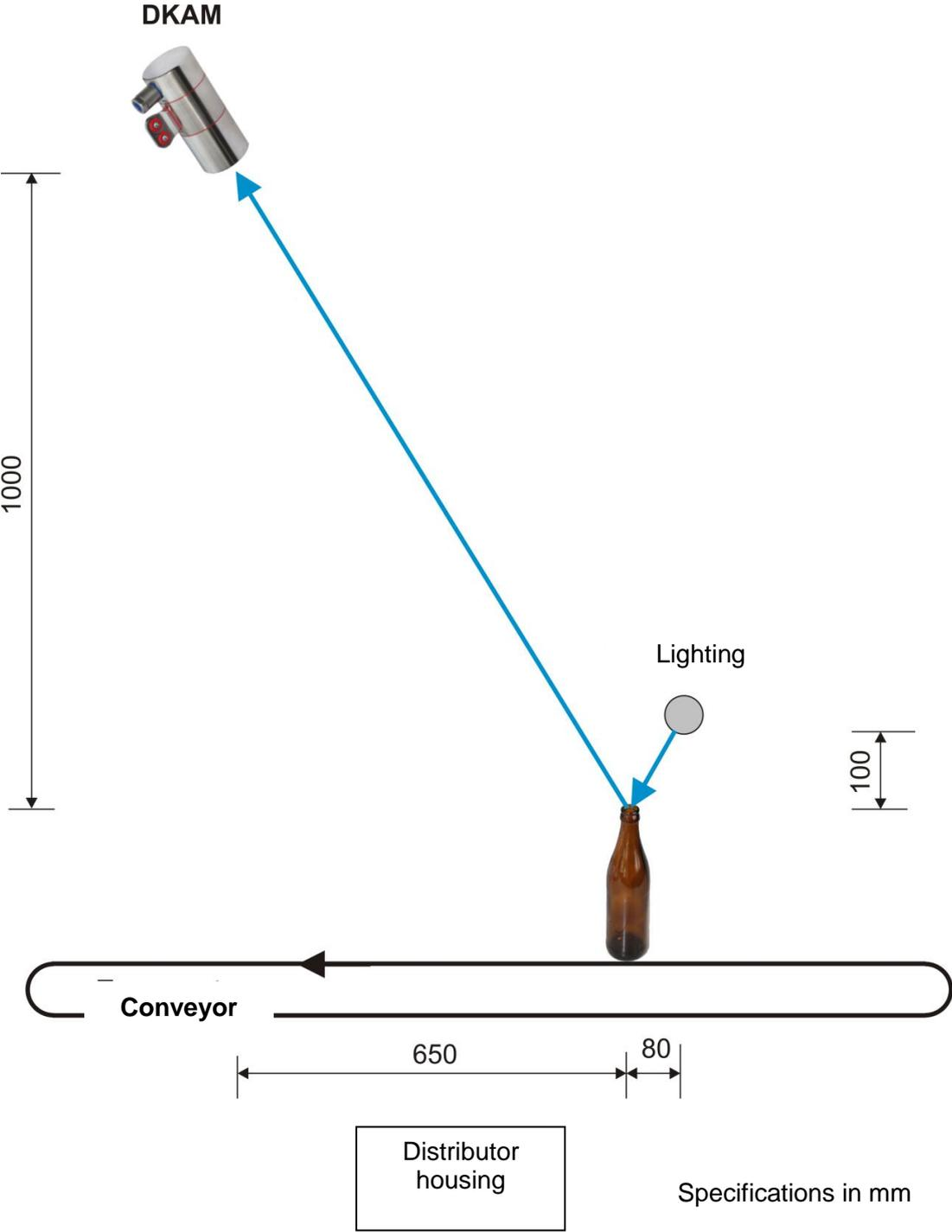
Fig.: Arrangement of DKAM and lighting. The distributor housing's placement must be adjusted to the system.
