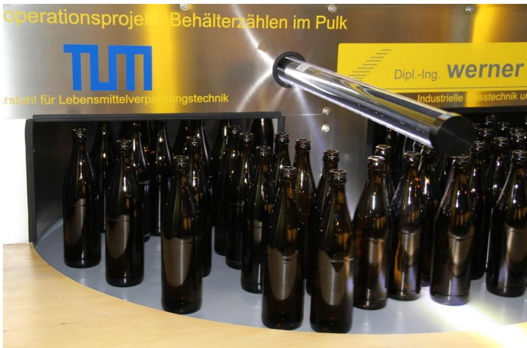
The containers (here: glass bottles) are conveyed in circles on a disk and are counted. The system distinguishes between open and closed bottles.
